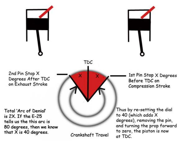
Figure 2 Timing Diagram
